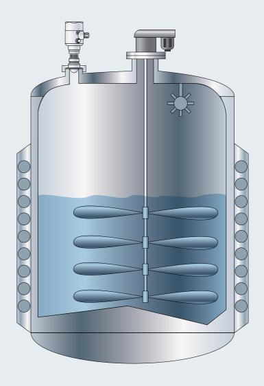
Measuring task: Level measurement Measuring range up to: 1.2 m Medium: Antibiotics, injection and infusion solutions, **Process temperature:** 50 to 150 °C Specific challenges: Changing product density, regular cleaning cycles, small vessels, response time and accuracy
