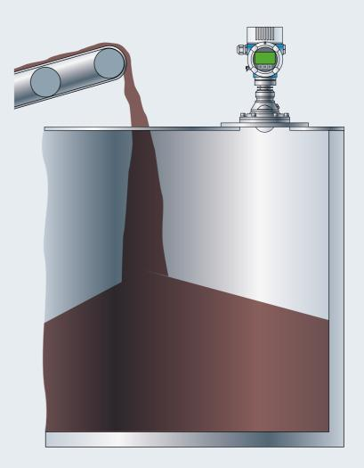
Measuring task: Level measurement Measuring range up to: 50m Medium: Stones, gravel and sand **Process temperature:** −40 bis 50 °C Weather conditions such as rain, snow and wind
