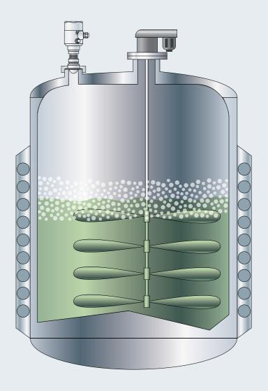
Measuring task: Level measurement **Process temperature:** Up to 150°C Specific challenges: Frequent foam
