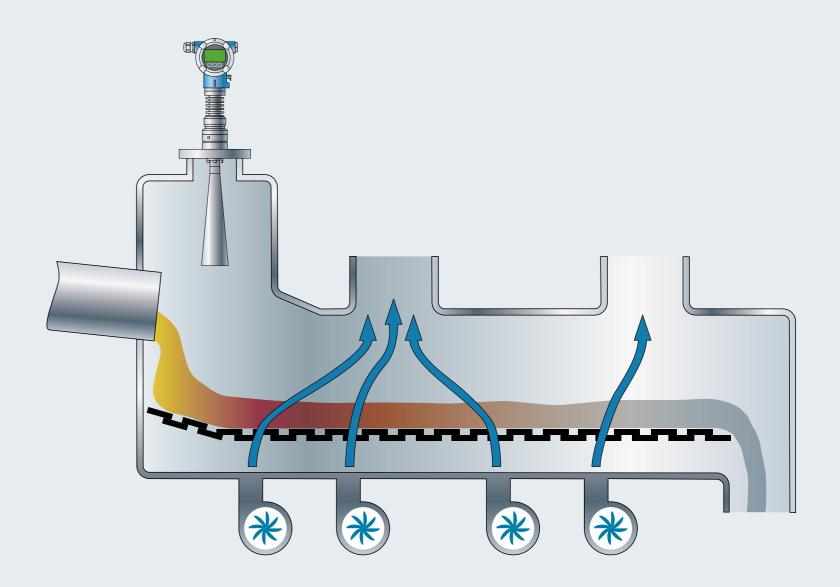
**Measuring task:** Level and pressure measurement Measuring point: Conveyor belt **Process temperature:** 0 to 1,500 °C Process pressure: 0 to 100 mbar High temperatures, dirt and buildup
