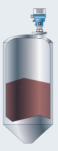
Measuring task: Level measurement and Medium: Stones, gravel and sand **Process temperature:** −40 bis 50 °C Extremely loud and dusty environments, abrasion
