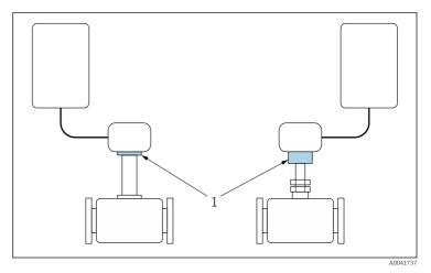
$\blacksquare 1$  Position of reference point for temperature measurement
