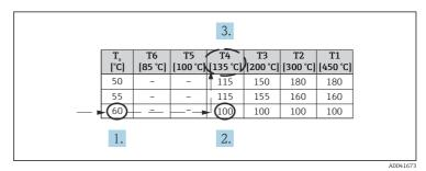
■ 2 Procedure for determining the temperature class and surface temperature
