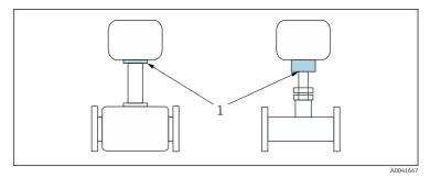
I Position of reference point for temperature measurement
