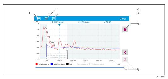
■ 32 Envelope curve display (sample) in SmartBlue for iOS
