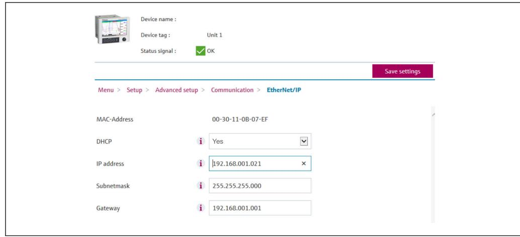
The screenshot shows a web-based configuration interface for network settings. At the top, there is a header with device information: Device name : (with a small icon), Device tag : Unit 1, and Status signal : ✓ OK. Below this is a 'Save settings' button. A navigation bar below the header shows the path: Menu > Setup > Advanced setup > Communication > EtherNet/IP. The main area contains the following configuration fields:
