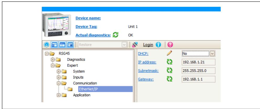
图 11 Network settings: confirm changes (DTM)
