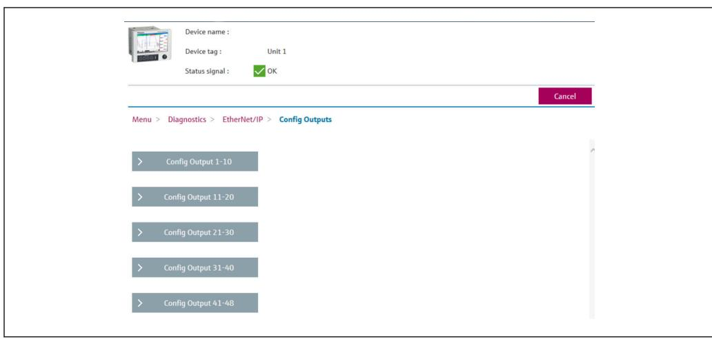
30 Visualization of Config Output submenu (web server)
