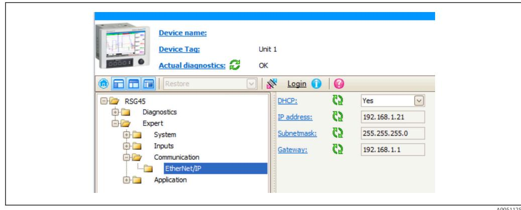
图 10 Network settings: DHCP enabled (DTM)
