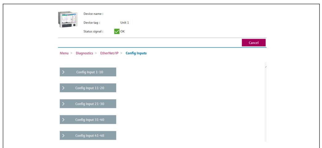
28 Visualization of Config Inputs submenu (web server)
