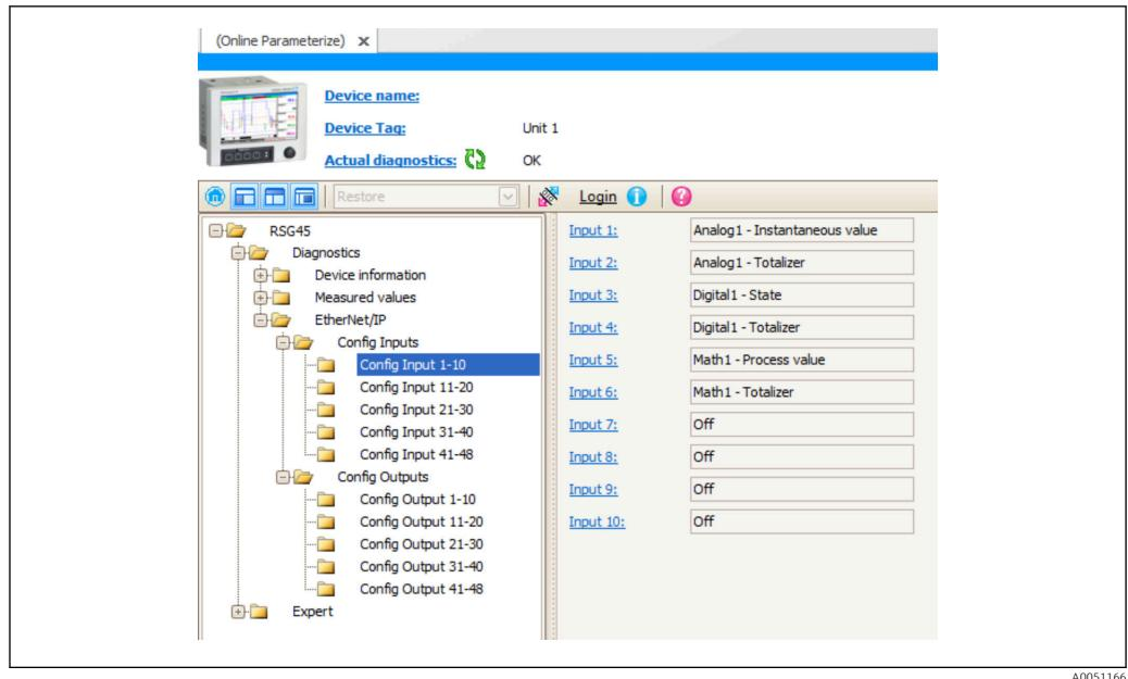
33 Visualization of Config Input 1-10 submenu (DTM)
