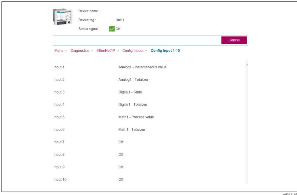
29 Visualization of Config Inputs submenu (web server)
