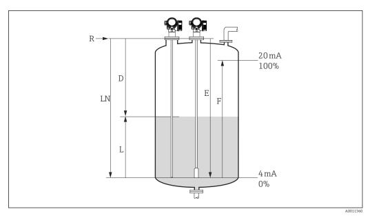
■ 23 Configuration parameters for level measurement in liquids
