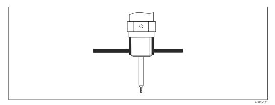
**₽** 5 Mounting with threaded connection; flush with the vessel ceiling
