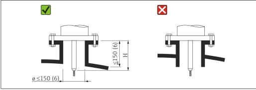
Length of the centering rod or the rigid part of the rope probe
