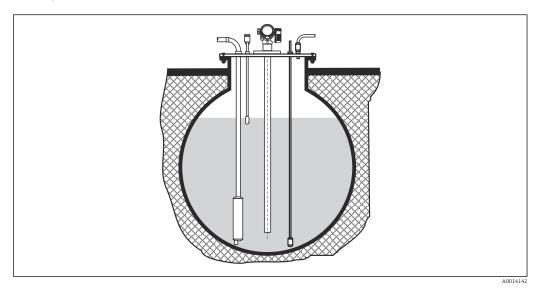
In the case of nozzles with large diameters, use FMP51 with a coax probe to avoid reflections at the nozzle wall.
