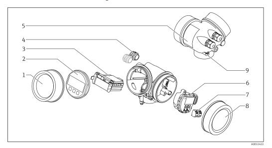
**₽** 2 Design of the electronics housing
