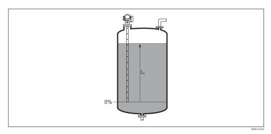
$\blacksquare$  33 Level in case of liquid measurements
