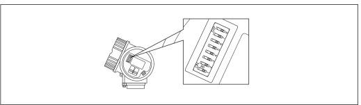
Address switch in the connection compartment
