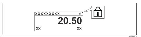
If hardware write protection is disabled, no option is displayed in the **Locking status** parameter. On the local display, the  $\blacksquare$  symbol disappears from in front of the parameters in the header of the operational display and in the navigation view.
