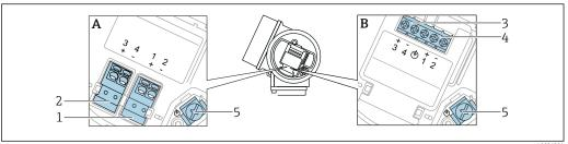
■ 10 Terminal assignment PROFIBUS PA / FOUNDATION Fieldbus
