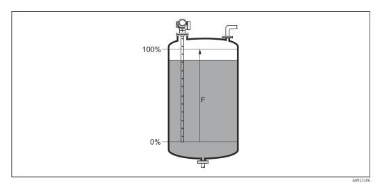
■ 32 Full calibration (F) for level measurements in liquids
