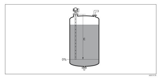
$\blacksquare$  31 Empty calibration (E) for level measurements in liquids
