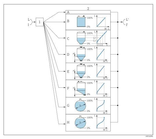
236 Linearization: Conversion of the level and, if applicable, interface into a volume or a weight; the conversion depends on the vessel shape
