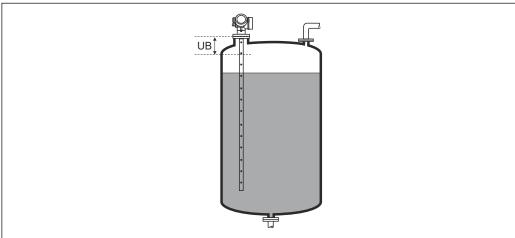
Blocking distance (UB) for liquid measurements
