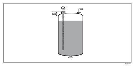
■ 35 Blocking distance (UB) for liquid measurements
