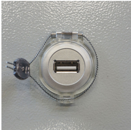
28 USB port sealed with sealing wire
