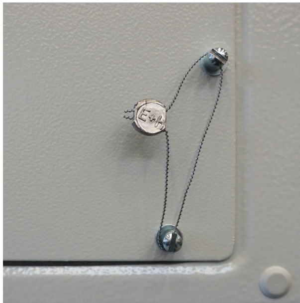
26 Screws sealed with sealing wire
