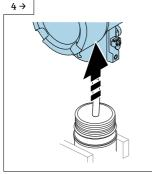
Carefully remove the housing from the sensor assembly, taking care not to damage the sensor cable.
