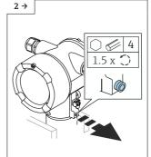
Housing lock for aluminum and stainless steel housing only. Not for plastic and hygienic housing.
