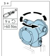
Using a suitable tool, unscrew the housing by applying significant force (> 60 Nm). This involves applying force several times in and against the screw direction; the snap ring is intentionally destroyed in the process. Do not damage the coating of the housing.
