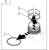
Replace the O-ring (2) and snap ring (1). In addition, replace the circlip (3) for the plastic and hygienic housing.
