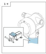
Protect the sensor assembly and housing from damage. Use a bench vise with braces.
