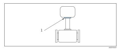
Position of reference point for temperature measurement
