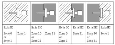
The device is designed for operation in explosive gas or explosive dust atmosphere as shown in the sketch above. In the event of potentially explosive gas-air and dust-air mixtures occurring simultaneously: Suitability requires further assessment.
