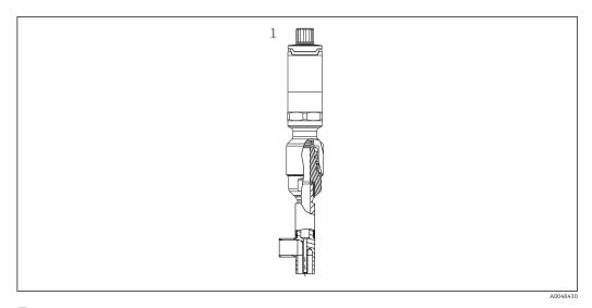
$\blacksquare$  4 Process connections for thermometer installation in pipes with small nominal diameters
