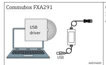
Connects Endress+Hauser field devices with a CDI interface (= Endress+Hauser Common Data Interface) and the USB port of a computer or laptop (Non-Ex area and Ex area).
