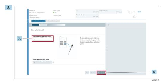
To read the calibration point data from the device, enter the calibration point index. Index 1 reads the latest calibration point.
