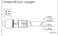
PVC cable,  $4 \times 0.34 \text{ mm}^2$  (22 AWG) with M12x1 coupling nut made of epoxy coated zinc; straight female connector type; screw plug; length 5 m (16.4 ft); IP69K
