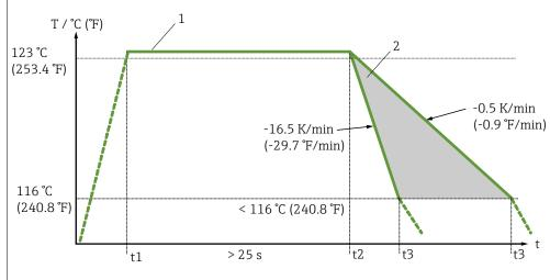
■ 10 Needed process temperature profile for self-calibration
