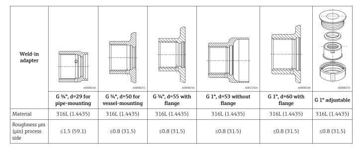
Maximum process pressure for the weld-in adapters:
