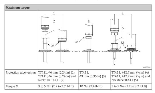
When connecting the device with the protection tube: only turn the hexagonal spanner flat on the bottom of the housing.
