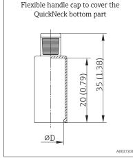
Diameter  $\varnothing$ D: 24 to 26 mm (0.94 to 1.02 in) Material: Thermoplastic polyolefin - elastomer (TPE), free from plasticizers
