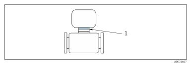
I Position of reference point for temperature measurement
