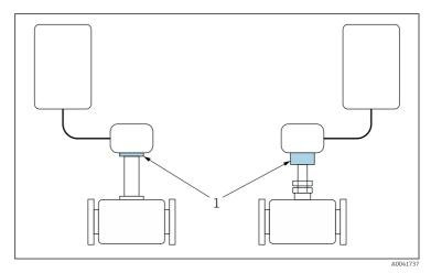
Position of reference point for temperature measurement
