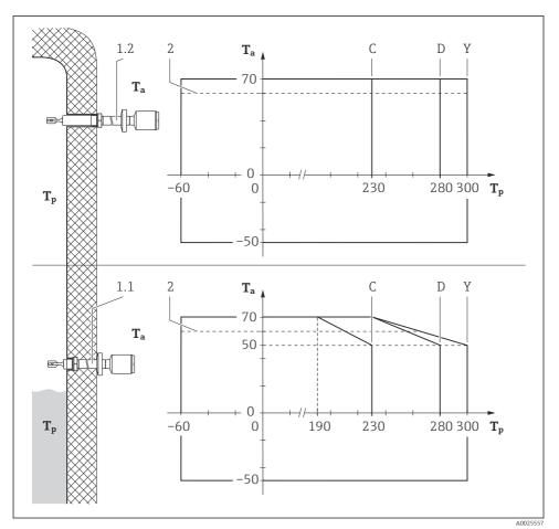
Device type FTL80, FTL81, Basic specification, Position 7 = C, D, Y
