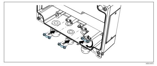
☑ 6 Installing the cable shield ground clamps (aluminum housing only)
