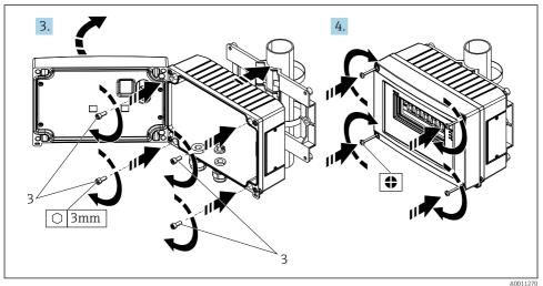
Attaching the indicator to the mounting plate
