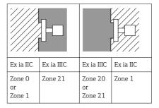
The device is designed for operation in explosive gas or explosive dust atmosphere as shown in the sketch above. In the event of potentially explosive gas-air and dust-air mixtures occurring simultaneously: Suitability requires further assessment.
