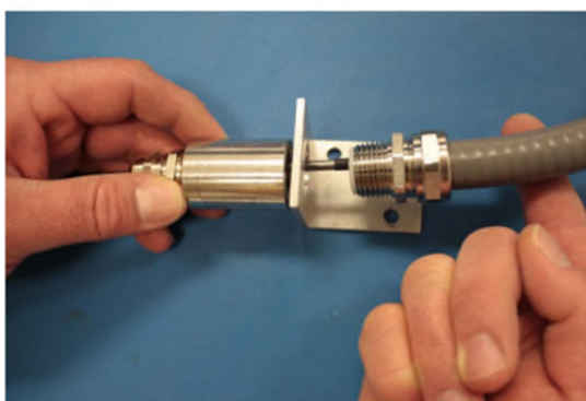
Figure 11. Feed oxygen probe through bracket opening and connect collar
