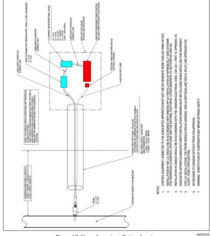
Figure 13. Hazard area installation drawing
