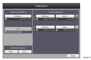
Figure 17. Calibration window with quick view buttons for a Raman Rxn2 Hybrid analyzer
