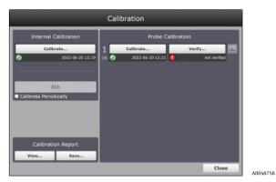
Figure 16. Calibration window with quick view buttons for a Raman Rxn2 single channel analyzer
