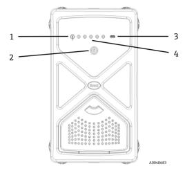
Figure 5. Front panel of a Raman Rxn2 four channel analyzer
