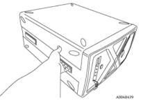
Figure 1. Raman Rxn2 integrated lifting handles
