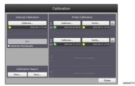
Figure 15. Calibration window with quick view buttons for a Raman Rxn2 four channel analyzer
