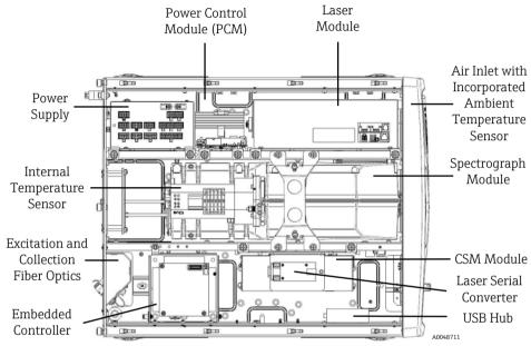
Figure 9. The interior of the Raman Rxn2 analyzer
