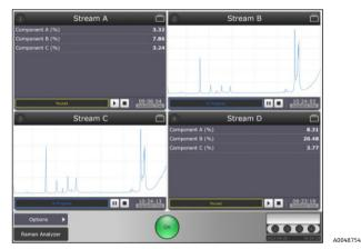
Figure 14. Raman RunTime main screen for a Raman Rxn2 four channel analyzer
