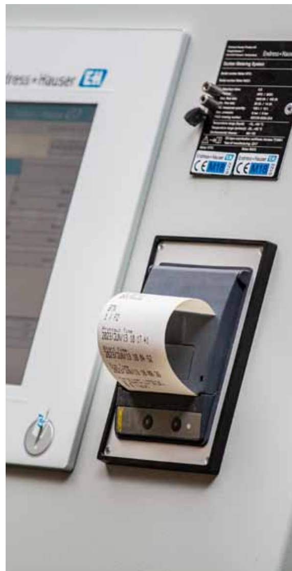
Bunker Metering Computer SBC600 with bunker metering ticket printed on an approved custody transfer printer
