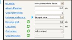
Go to the **LRC Mode** parameter and select the **Compare with level device** option.
