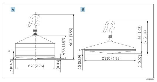
A Ø70 mm (2.76 in) 316L conical displacer
