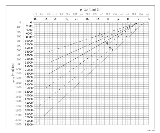
I6 Lateral shift of displacer according to measurement range
