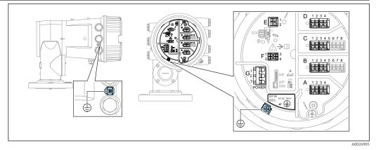
11 Terminal compartment (typical example) and ground terminals
