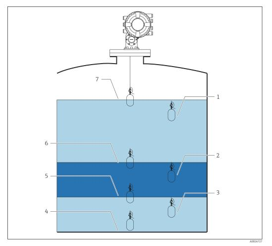
Image: A NMS8x with standard level, I/F x 2, Tank bottom and spot density x 3 measurement
