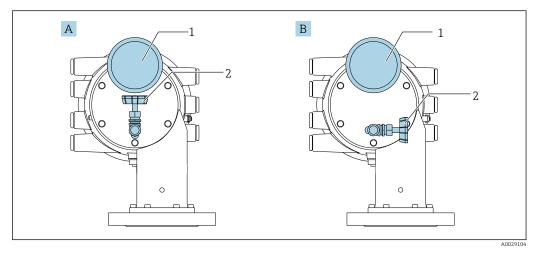
28 Mounting position of relief valve and pressure gauge
