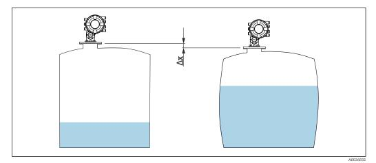
$\blacksquare$  24 Movement  $\Delta x$  of the tank reference height due to the bulging of the tank shell caused by hydrostatic pressure
