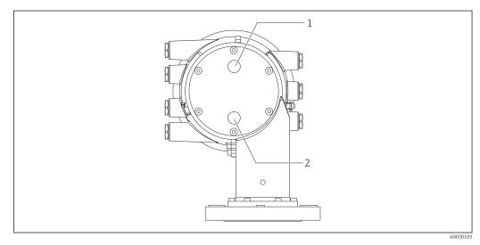
■ 31 Holes for cleaning nozzle and gas purging nozzle
