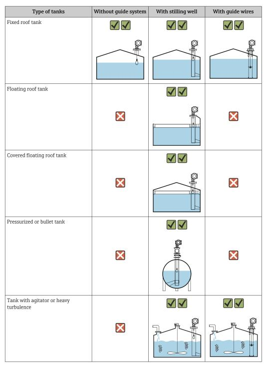
• A stilling well is required in a floating roof tank and a covered floating roof tank.
