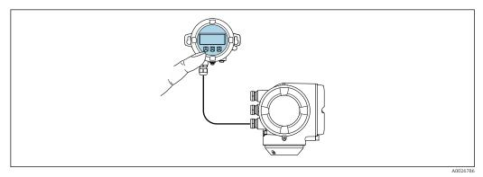
₹ 36 Operation via remote display and operating module DKX001
