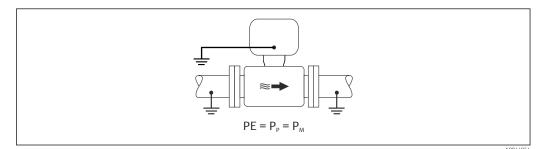
► Connect the connection housing of the transmitter or sensor to ground potential by means of the ground terminal provided for this purpose.
