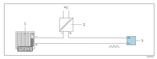
$\blacksquare$  11 Connection example for pulse/frequency output (passive)
