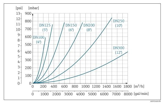
34 Pressure loss DN 100 to 300 (4 to 12") for order code for "Design", option C "Fixed flange, constricted measuring tube", 0 x DN inlet/outlet runs"
