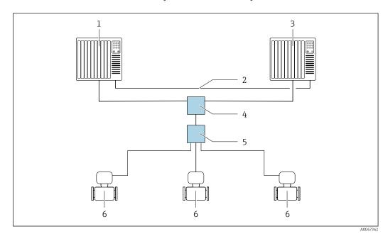
■ 22 Example of the layout of a redundant system (S2): star topology
