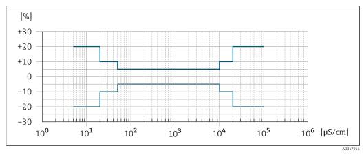
■ 32 Measured error (optional: order code for "Calibrated conductivity measurement", option CW)
