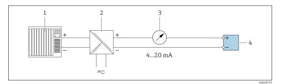
■ 10 Connection example for 4-20 mA current output (passive)
