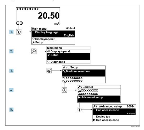
The number of submenus and parameters can vary depending on the device version. Certain submenus and parameters in these submenus are not described in the Operation Instructions. Instead a description is provided in the Special Documentation for the device (→ "Supplementary documentation" section).
