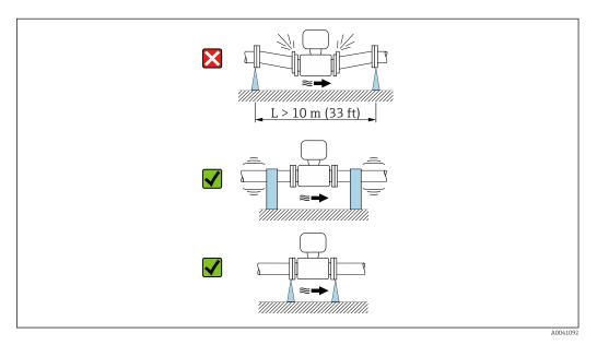
Information on the measuring system's resistance to vibration and shock  $\rightarrow \stackrel{\triangle}{=} 206$
