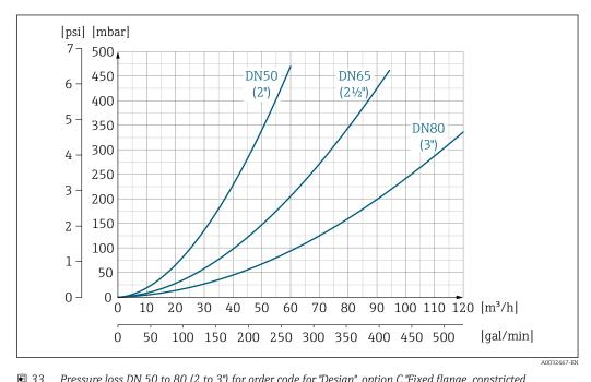
$\blacksquare$  33 Pressure loss DN 50 to 80 (2 to 3") for order code for "Design", option C "Fixed flange, constricted measuring tube", 0 x DN inlet/outlet runs"
