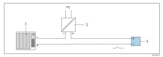
■ 12 Connection example for switch output (passive)
