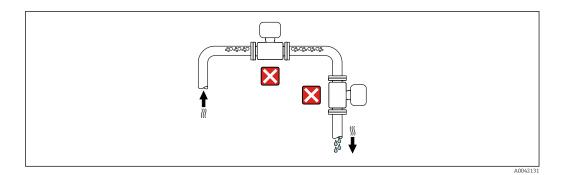
The device should ideally be installed in an ascending pipe.
