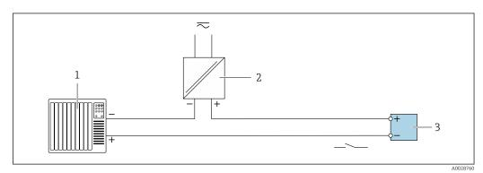
14 Connection example for switch output (passive)
