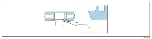
■ 5 Thermal insulation with not isolated extended neck
