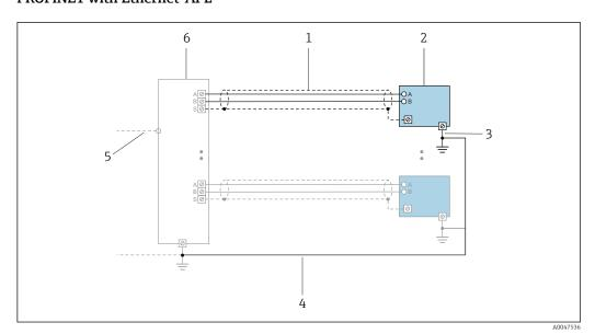
$\blacksquare$  10 Connection example for PROFINET with Ethernet-APL
