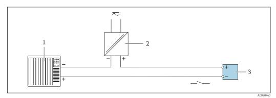
15 Connection example for switch output (passive)
