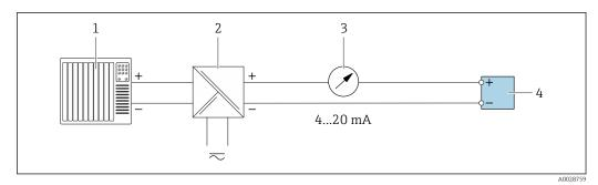
■ 13 Connection example for 4-20 mA current output (passive)
