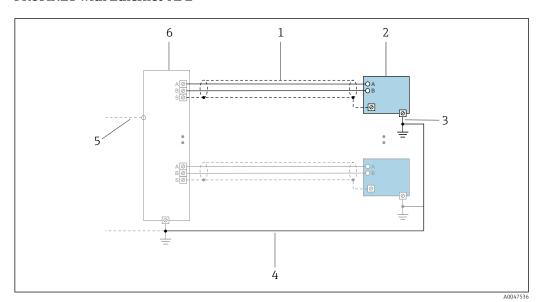
11 Connection example for PROFINET with Ethernet-APL
