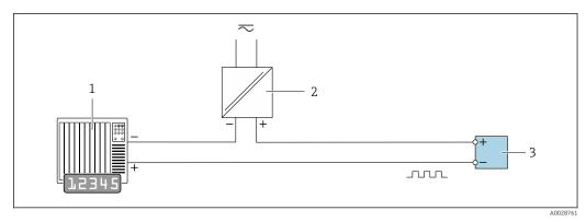
■ 14 Connection example for pulse/frequency output (passive)
