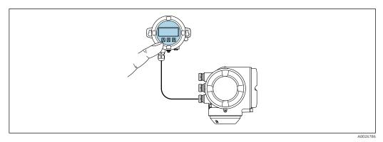
35 Operation via remote display and operating module DKX001
