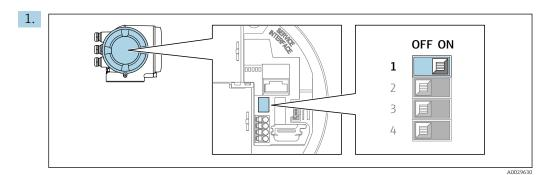
Setting the write protection (WP) switch on the main electronics module to the **ON**
