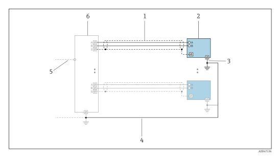
10 Connection example for PROFINET with Ethernet-APL
