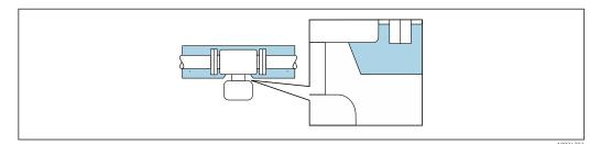
**■** 5 Thermal insulation with not isolated extended neck
