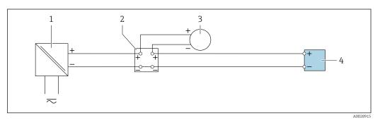
■ 16 Connection example for 4 to 20 mA current input
