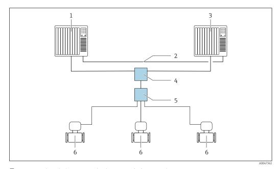
■ 24 Example of the layout of a redundant system (S2): star topology
