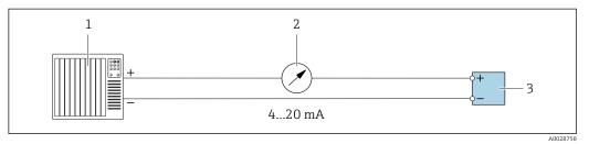
■ 12 Connection example for 4-20 mA current output (active)
