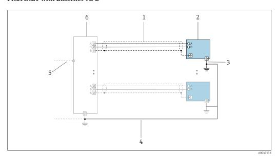
I1 Connection example for PROFINET with Ethernet-APL
