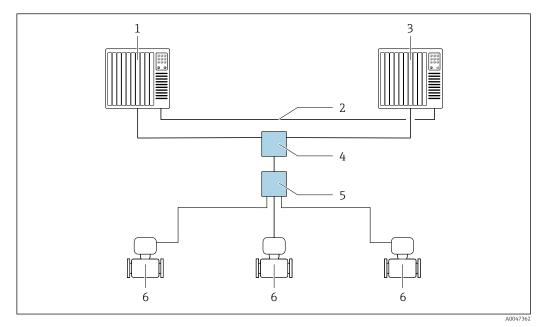
■ 25 Example of the layout of a redundant system (S2): star topology
