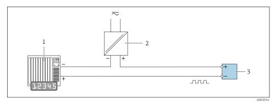
■ 14 Connection example for pulse/frequency output (passive)
