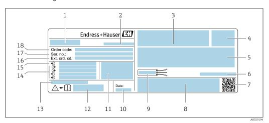
■ 3 Example of a transmitter nameplate
