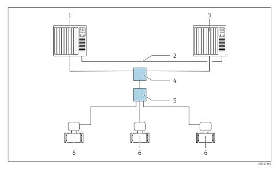
■ 33 Example of the layout of a redundant system (S2): star topology
