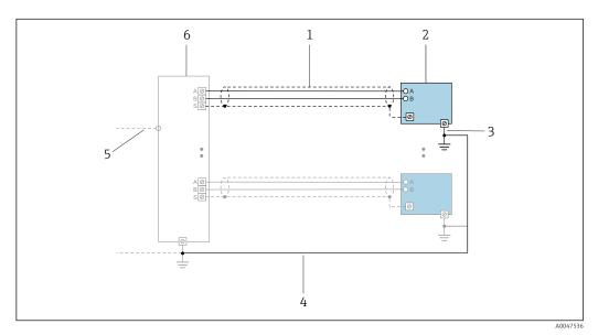
$\blacksquare$  18 Connection example for PROFINET with Ethernet-APL
