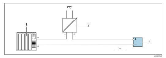
**₽** 22 Connection example for switch output (passive)
