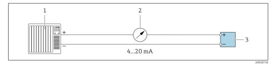
■ 19 Connection example for 4-20 mA current output (active)
