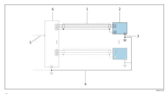
■ 15 Connection example for PROFINET with Ethernet-APL
