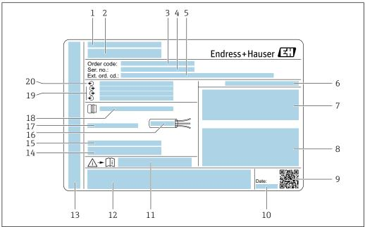
■ 4 Example of a transmitter nameplate
