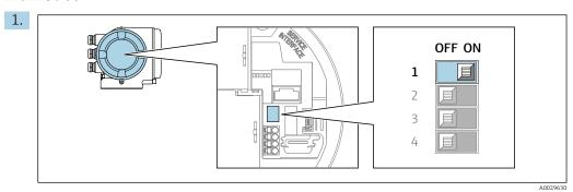
Setting the write protection (WP) switch on the main electronics module to the  ${\bf ON}$  position enables hardware write protection.
