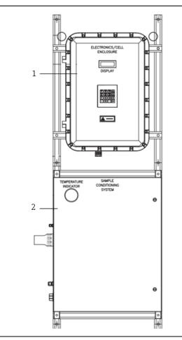
The analyzer system on a panel consists of the following and is designed for exterior mounting near the sample extraction point or inside a shelter:
