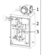
The enclosed analyzer system with optional heater consists of the following and is typically used for exterior mounting near the sample extraction point.
