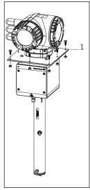
1 Optional mounting plate allows top-mounting of the J22 analyzer within user-supplied enclosure (not shown)
