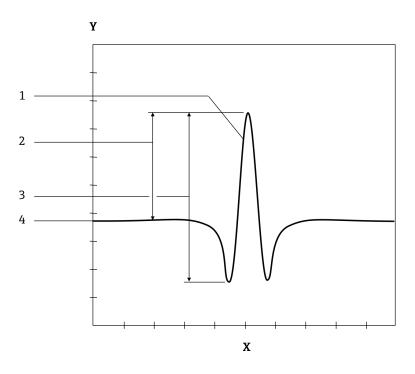
$\blacksquare$  2-3: Simple normalized 2f signal; analyte concentration proportional to the peak height or the peak-to-peak height, depending on the algorithm used
