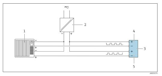
🛃 18 Connection example for double pulse output (passive)
