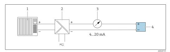
■ 14 Connection example for 4-20 mA current output (passive)
