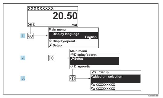
29 Navigation to "Setup" menu using the example of the local display
