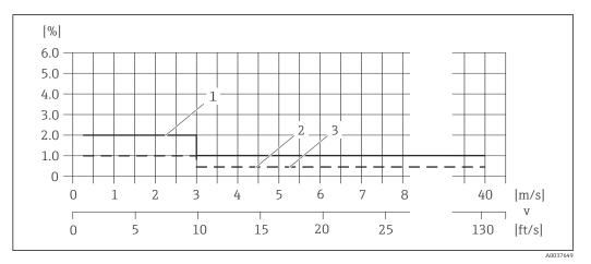
35 Maximum measurement error (volume flow) in % of reading
