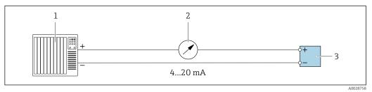
■ 13 Connection example for 4-20 mA current output (active)
