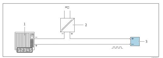
15 Connection example for pulse/frequency output (passive)
