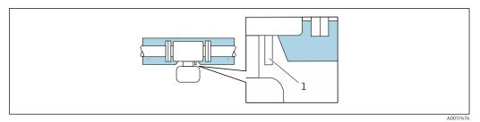
☑ 7 Thermal insulation with free extended neck and pressure measuring cell
