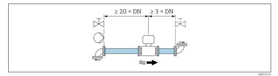
If a single-path version: Minimum inlet and outlet runs with various flow obstructions. For order code for "Flow calibration", option A "1 %".
