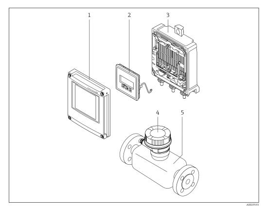
■ 1 Important components of a measuring device
