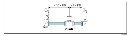
5 Two-path version: minimum inlet and outlet runs with various flow obstructions For order code for "Flow calibration", option A "1 %" ".
