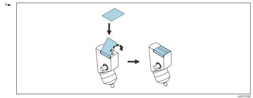
2. Equip all sensors used with coupling foil!
