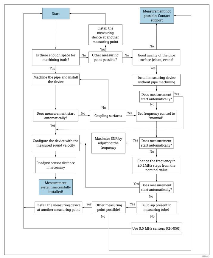
6.3 Workflow for mounting the sensors
