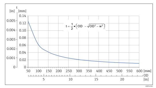
I Material to be removed depending on the external pipe diameter
