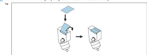
1. Fold the foil over the slightly angled surface of the sensor body.
