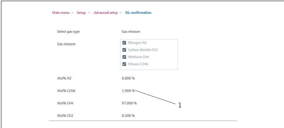
3 Web browser view of the configuration of the natural gas composition in the SIL mode
