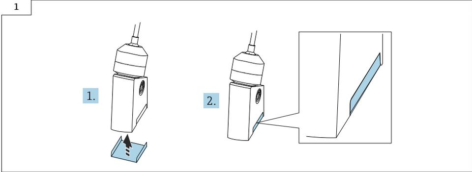
► Fold the foils onto the slightly inclined surface of the sensor bodies.
