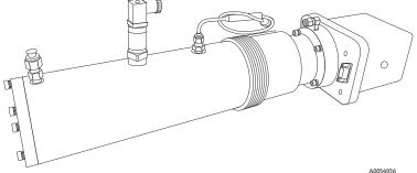
Figure 9. Removed measurement cell with pressure sensor oriented up
