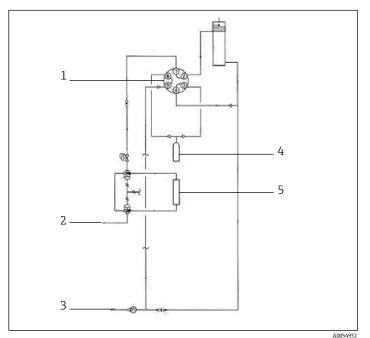
Figure 6. Flow diagram of differential sample system with permeation tube validation
