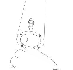
Figure 12. Removing excess seal tape from inside measurement cell
