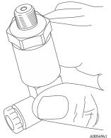
Figure 13. Replacing the seal tape
