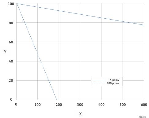
Figure 22. Predicted scrubber lifetime based on average H<sub>2</sub>S load
