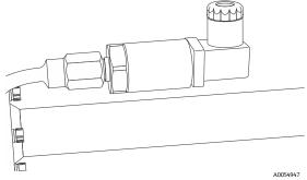
Figure 21. Newly installed pressure sensor positioning
