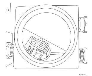
Figure 2. AC connection terminal block for enclosure heater
