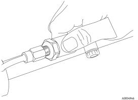
Figure 20. Replacing the pressure sensor
