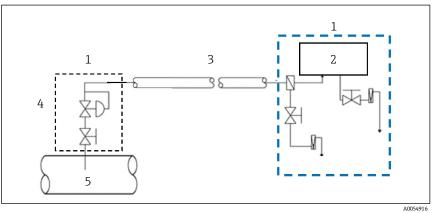
Figure 1. Sample regulators at probe
