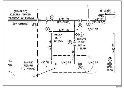
2. Open the cell supply and cell return shut-off valves. Refer to your as-built drawings for exact locations.
