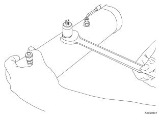
Figure 10. Removing the old pressure sensor
