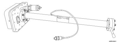
Figure 16. Removed 0.8 m measurement cell with pressure sensor face up
