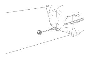
Figure 11. Removing excess seal tape from flange
