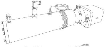
Figure 15. New pressure sensor installed
