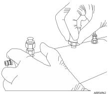
Figure 14. Replacing the pressure sensor
