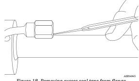
Figure 18. Removing excess seal tape from flange
