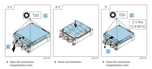
The device does not display the remaining capacity of the external batteries. The value on the display refers exclusively to the batteries fitted internally. If internal and external batteries are connected, the external batteries are used first of all, and then the internal batteries are used.
