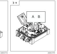
Open the connection compartment cover. ► Open the display module.
