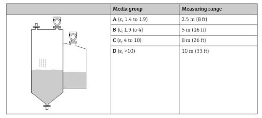
Process connection MNPT/G 1½, NEUMO BioControl D50, 80 GHz in storage vessel
