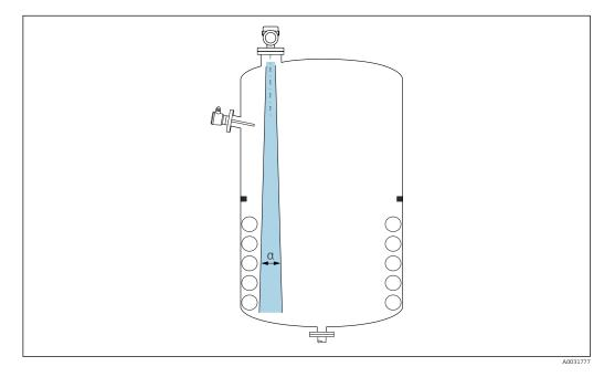
Avoid internal fittings (point level switches, temperature sensors, struts, vacuum rings, heating coils, baffles etc.) inside the signal beam. Pay attention to the beam angle  $\alpha$ .
