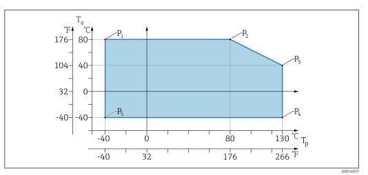
$\blacksquare$  9 Ambient temperature  $T_a$  depending on the process temperature  $T_p$
