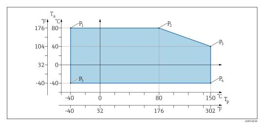
$\blacksquare$  8 Ambient temperature  $T_a$  depending on the process temperature  $T_p$
