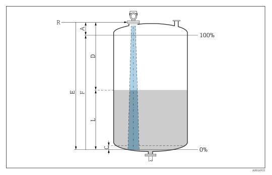
**■** 5 Configuration parameters for level measurement in liquids
