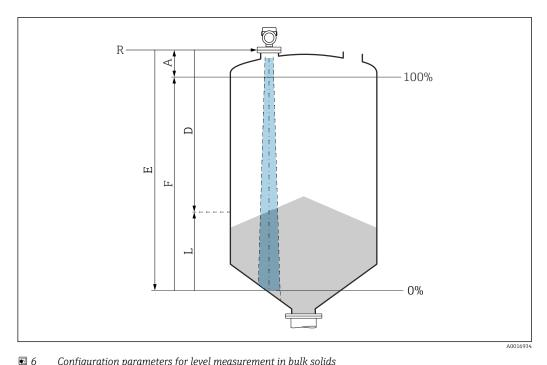
Configuration parameters for level measurement in bulk solids
