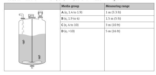
Process connections TriClamp 1½, TriClamp 2, 80 GHz in vessel with agitator
