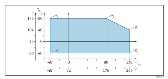
lacksquare 11 Ambient temperature  $T_a$  depending on the process temperature  $T_p$
