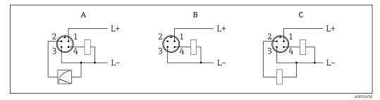
*A* 1 x PNP switch and analog output (default setting)
