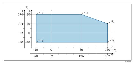
$\blacksquare$  10 Ambient temperature  $T_a$  depending on the process temperature  $T_p$
