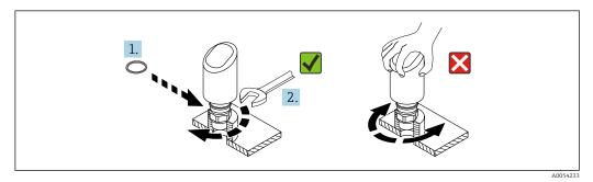
■ 2 Screwing in the device
