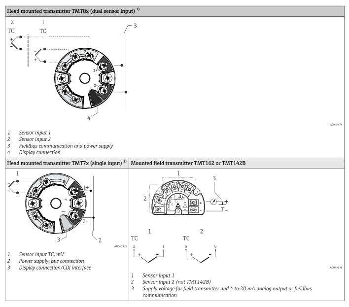
1) Fitted with spring terminals if screw terminals are not explicitly selected or a dual sensor is installed.
