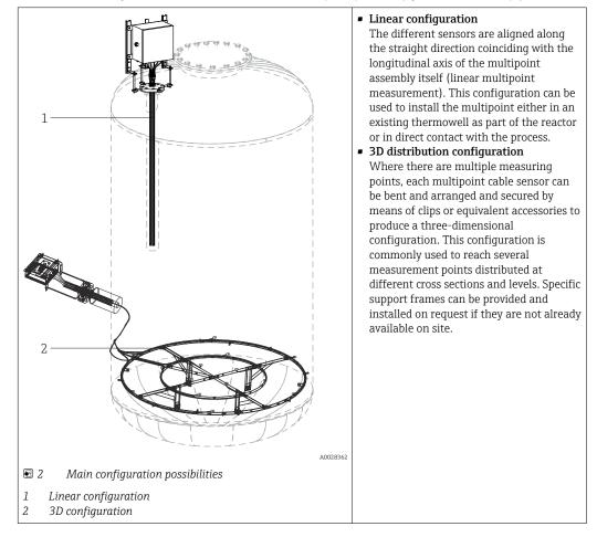
The modular multipoint thermometer is characterized by the following possible main configurations:
