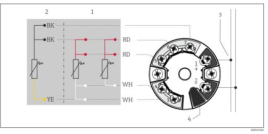
■ 5 Head mounted transmitter TMT8x (dual input)
