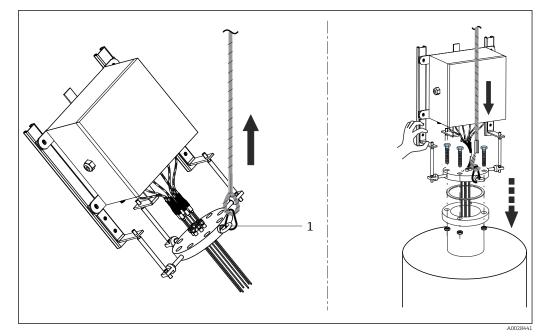
■ 10 Multipoint thermometer installation in a reactor nozzle via flange process connection.
