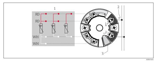
Head mounted transmitter TMT7x or TMT31 (single input)
