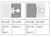
The device is designed for operation in explosive gas or explosive dust atmosphere as shown in the sketch above. In the event of potentially explosive gas-air and dust-air mixtures occurring simultaneously: Suitability requires further assessment.
