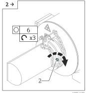
► Using an Allen key, tighten the screws (2) on the cover.
