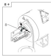
Move the lock pin (8) out of the "OFF" position and into the parking position.
