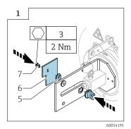
► Tighten 2 x Allen screws (7) (AF3) to secure the cover plate (6) and the plain bearing bushing (5).
