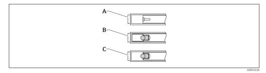
Α Fix the capsule with thread in an appropriate device and turn the slidable source holder.
