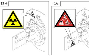
If necessary, attach the "Highly radioactive" adhesive label to the source container.
