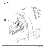
Check whether the lock pin (8) is inserted in the OFF position.
