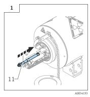
► Insert the complete slidable source holder (11) along with the protection pipe into the source container.
