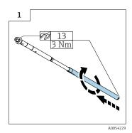
Using a torque wrench (AF13) and open-ended wrench (AF13), tighten the source holder combination to 3 Nm.
