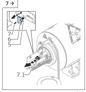
► Release 2 x Allen screws (7) (AF3) to remove the cover plate (6) and the plain bearing bushing (5).
