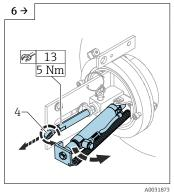
Unscrew the complete thrust rod (4) (AF13).
