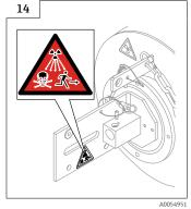
If necessary, attach the "Highly radioactive" adhesive label to the source container.
