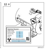
► Turn the slidable source holder to unscrew it from the protection pipe (12) ► Attach the "Gamma Source" adhesive nameplate to the slidable source holder.
