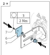
➤ Tighten 2 x Allen screws (7) (AF3) to secure the cover plate (6) and the plain bearing bushing (5).
