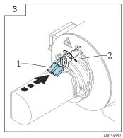
Attach padlock (1) and sealing wire with seal (2).
