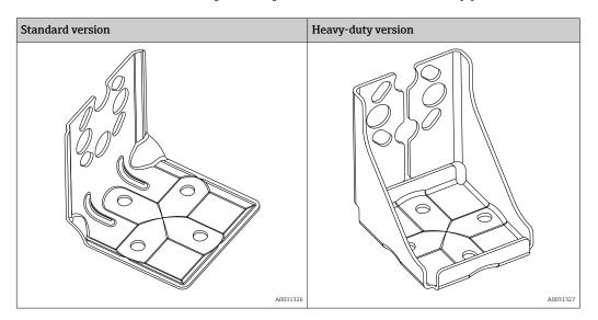
The standard mounting bracket version is **not** suitable for use in an application subject to vibrations.
