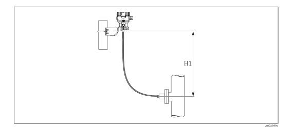
The maximum height difference depends on the density of the fill fluid and the lowest pressure that is permitted to occur at the diaphragm seal (empty vessel). See illustration below. The following diagram shows the maximum installation height above the lower diaphragm seal for vacuum applications.
