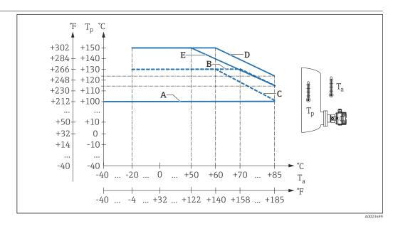
A, B C, D and E, see following section.  $T_a$  = Ambient temperature.  $T_p$  = Process temperature
