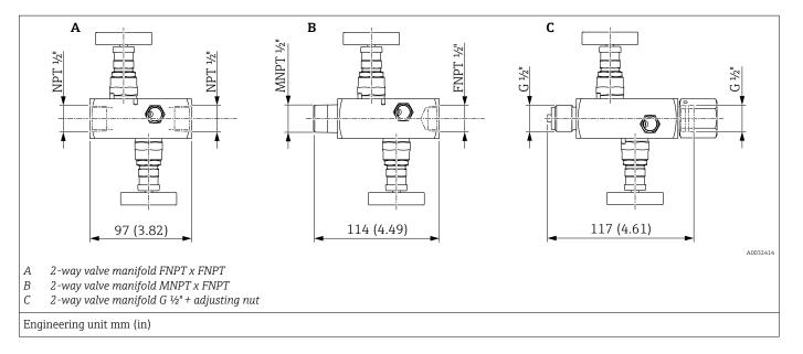
2-way valve manifolds in 316L or AlloyC can be ordered
