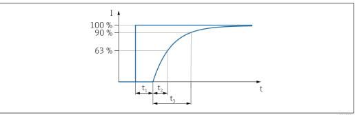
Step response time = dead time  $(t_1)$  + time constant T90  $(t_3)$  according to IEC62828-1
