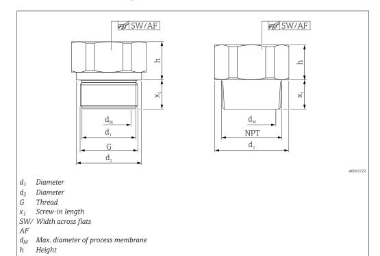
Unit mm (in). Left: thread ISO228, right: thread ASME Schematic diagram, the design may differ.
