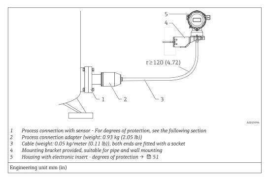
Degree of protection for the process connection and sensor with the use of
