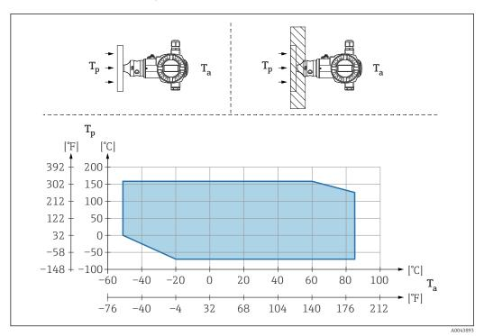
*T<sub>a</sub>* Ambient temperature at transmitter
