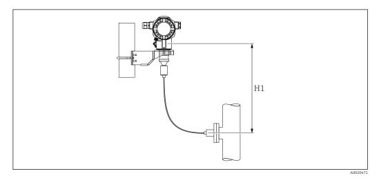
The maximum height difference depends on the density of the fill fluid and the smallest ever pressure that is permitted to occur at the diaphragm seal (empty vessel), see the diagram below. The following diagram depicts the maximum installation height above the diaphragm seal for vacuum applications.
