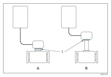
$\blacksquare$  1 Position of reference point for temperature measurement
