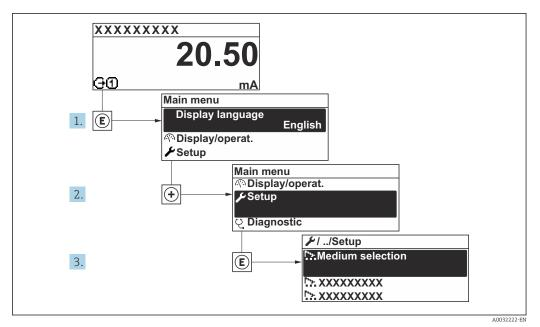
48 Navigation to "Setup" menu using the example of the local display
