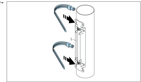
$\blacksquare$  17 Position the sensor holder and fit the strapping bands.
