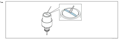
■ 30 Coating the contact surfaces of the sensor with coupling gel (if there is no coupling pad)
