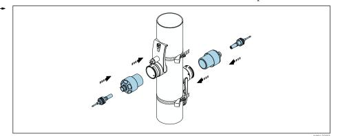
5. Insert the sensor cable into each individual sensor until the end stop.
