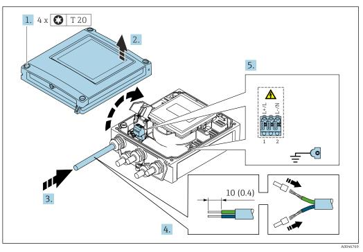
38 Connecting the supply voltage and 0-20 mA/4-20 mA HART with additional outputs and inputs
