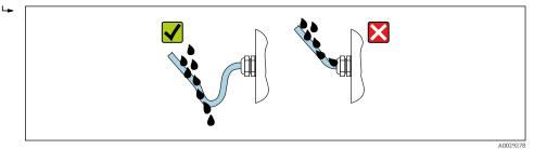
5. The cable glands supplied do not ensure housing protection when not in use. They must therefore be replaced by dummy plus corresponding to the housing protection.
