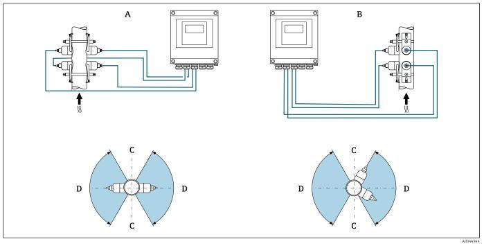
E 6 Two-path measurement: examples of the horizontal arrangement of the sensor sets at a measuring point
