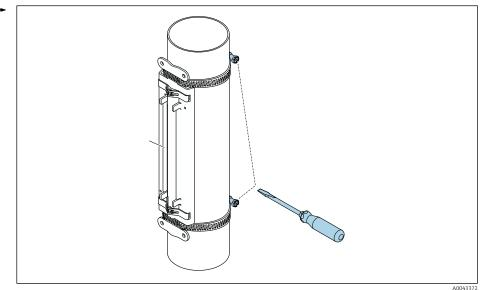
■ 18 Tighten the tensioning screws of the strapping bands.
