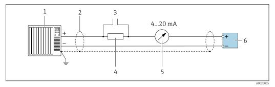
39 Connection example for 4 to 20 mA HART current output (active)
