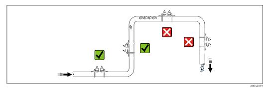
To prevent measuring errors arising from accumulation of gas bubbles in the measuring pipe, avoid the following mounting locations in the piping:
