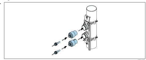
**I** 34 *Mounting the sensors and connecting the sensor cables*
