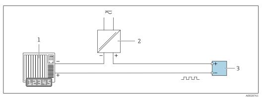
■ 40 Connection example for pulse/frequency output (passive)
