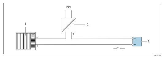
■ 41 Connection example for switch output (passive)
