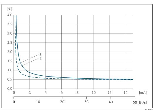
Example of max. measurement error (volume flow)
