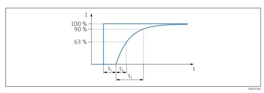
Step response time = dead time  $(t_1)$  + time constant T90  $(t_3)$  according to IEC62828-1
