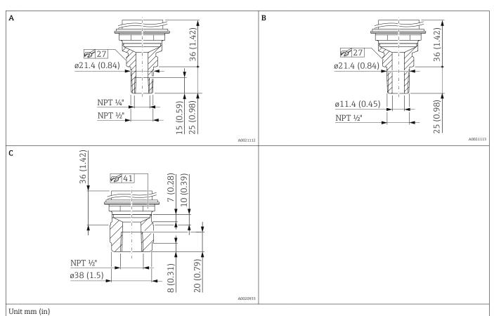
Thread ASME B1.20.1, internal membrane, standard (without diaphragm seal)
