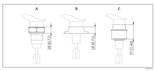
■ 29 Maximum height specification for the process connections. Unit of measurement mm (in)
