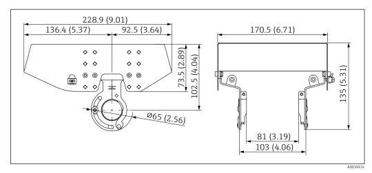
■ 40 Weather protection cover for dual compartment housing. Unit of measurement mm (in)
