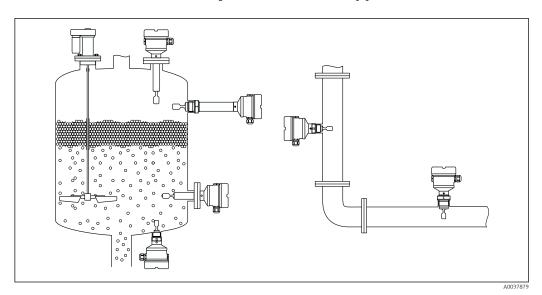
**₽** 7 Installation examples for a vessel, tank or pipe
