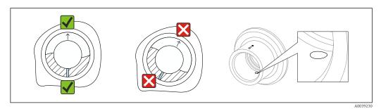
$\blacksquare$  18 Weld-in adapter with leakage hole
