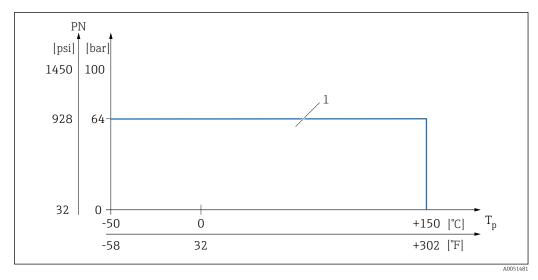
1 PN: 64 bar (928 psi) for a maximum of 150  $^{\circ}$ C (302  $^{\circ}$ F), refer to "Process connections" section for exceptions
