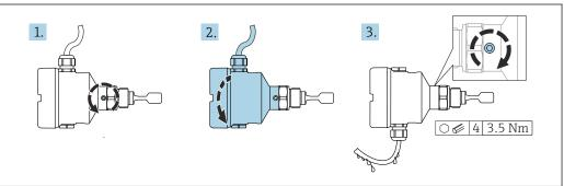
$\blacksquare$  15 Housing with external locking screw and drip loop
