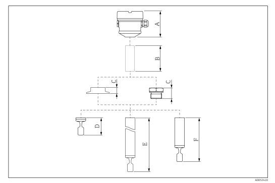
$\blacksquare$  21 Components to determine the device height
