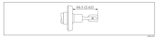
■ 34 DIN11851 pipe union. Unit of measurement mm (in)
