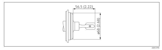
₹ 35 Varivent N pipe DN65-162 PN25. Unit of measurement mm (in)
