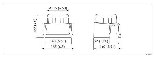
■ 41 Protective cover for aluminum single compartment housing. Unit of measurement mm (in)
