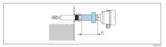
■ 25 Ex d glass feedthrough for pipe extensions
