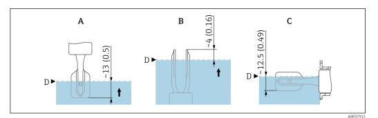
₩ 5 Typical switch points. Unit of measurement mm (in)
