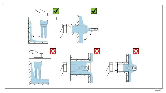
$\blacksquare$  10 Installation examples for a highly viscous process medium
