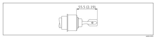
■ 33 Flush-mounted tank connection. Unit of measurement mm (in)
