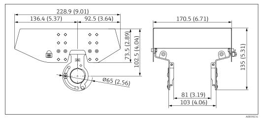
37 Protective cover for aluminum dual compartment housing. Unit of measurement mm (in)
