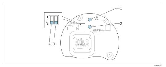
■ 35 Operating keys and DIP switch on FEL60H electronic insert
