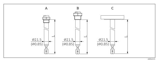
🖻 25 Pipe extension (sensor length L). Unit of measurement mm (in)
