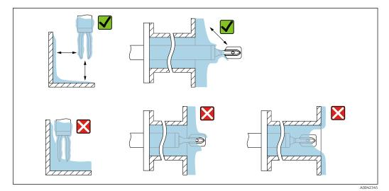
Installation examples for a highly viscous process medium
