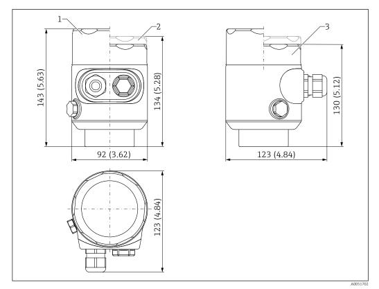
Dimensions of single-compartment housing, 316 L, hygienic. Unit of measurement mm (in) 20
