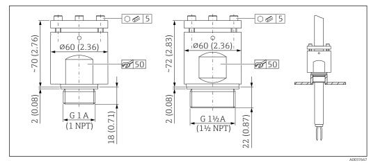
■ 40 High pressure sliding sleeves. Unit of measurement mm (in)
