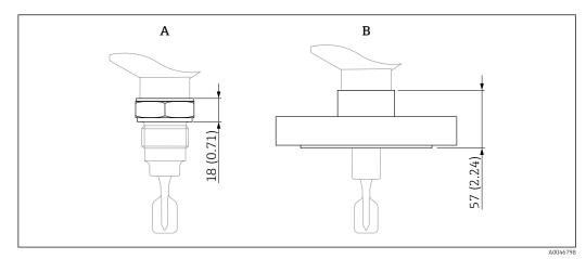
🖻 27 Maximum height specification for the process connections
