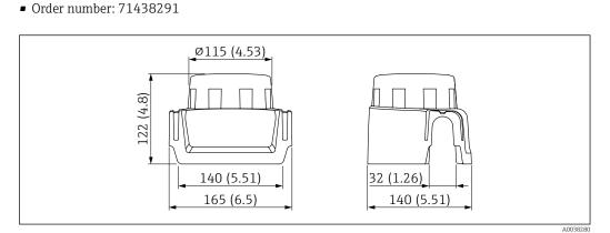
🛃 38 Protective cover for single compartment housing, aluminum or 316L. Unit of measurement mm (in)
