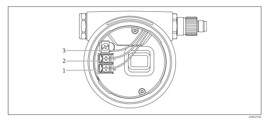
₽ 2 Connection terminals and ground terminal in the connection compartment
