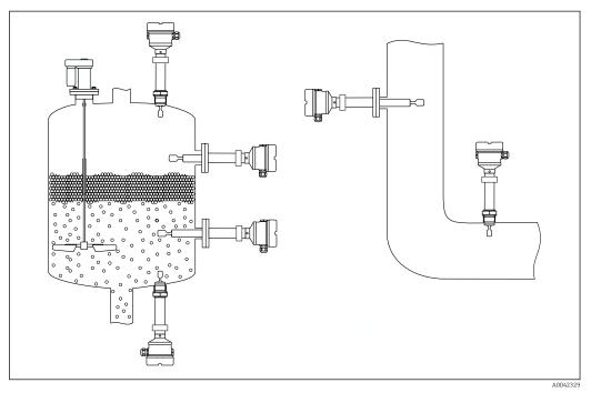
Installation examples for a vessel, tank or pipe
