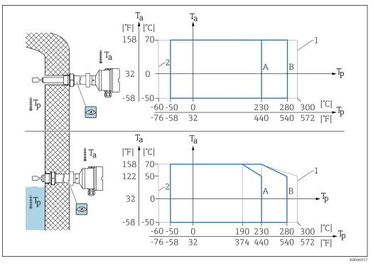
$\blacksquare$  17 Permitted ambient temperature  $T_a$  at the housing as a function of the process temperature  $T_p$  in the vessel
