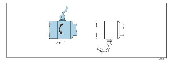
■ 13 Housing without locking screw with drip loop
