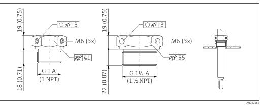
$\blacksquare$  39 Sliding sleeves for unpressurized operation  $p_e = 0$  bar (0 psi). Unit of measurement mm (in)
