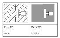
The device is designed for operation in explosive gas or explosive dust atmosphere as shown in the sketch above. In the event of potentially explosive gas-air and dust-air mixtures occurring simultaneously: Suitability requires further assessment.
