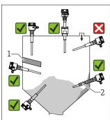
Installation in any direction in the bulk solids silo
